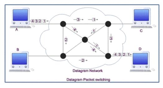
The above diagram approach is used to deliver 4 packets from station A to station D. All the four packets belong to same message but they may travel via different paths to reach the destination.
