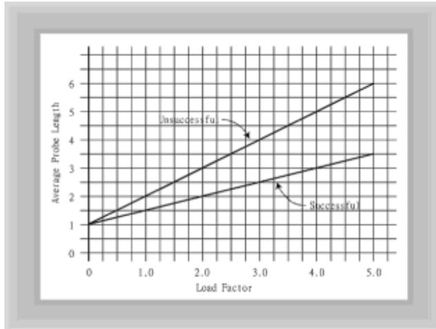
**Figure 11.14:** Separate-chaining performance
