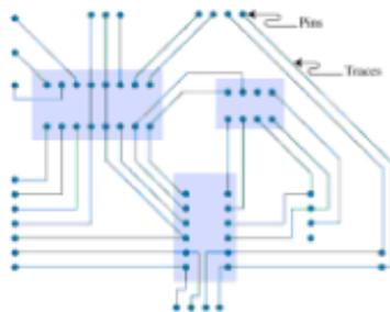
**Figure 13.4:** pins and traces on a circuit board
