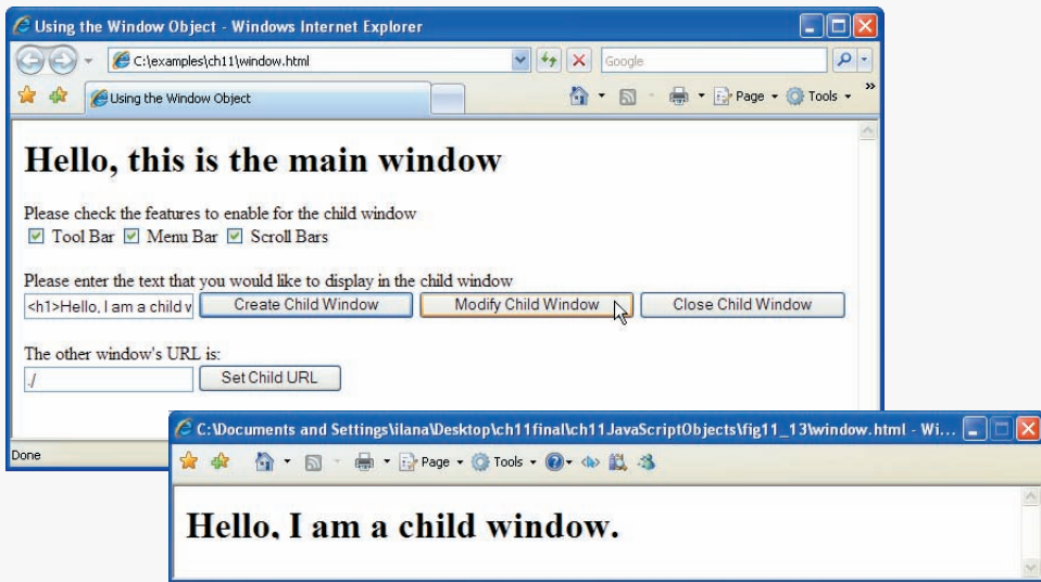
Fig. 11.13 | Using the window object to create and modify child windows. (Part 4 of 4.)
