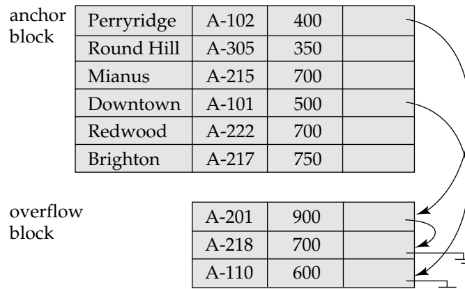
Figure 11.14 Anchor-block and overflow-block structures.
